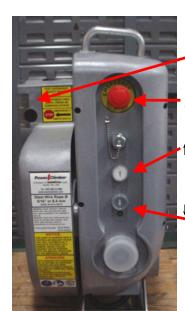
Overspeed Brake Test Button
