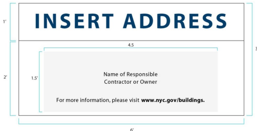
FIGURE 3301.9.2.1(1) SIDEWALK SHED PARAPET PANEL LAYOUT
