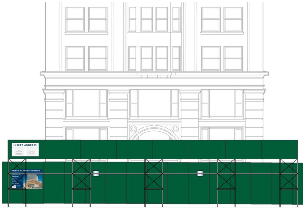
FIGURE 3301.9.2.2 PANEL POSTING ELEVATION DIAGRAM
